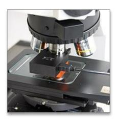
The Nanosurf LensAFM is an atomic force microscope (AFM) that may be used in conjunction with almost any upright optical microscope or optical profilometer. The combined LensAFM/optical platform provides a complementary imaging system that greatly extends the resolution and measuring capabilities of these individual instruments.
