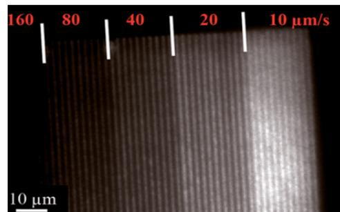
Line widths in liquid can be adjusted by variation of speed, pressure and force<sup>[3]</sup>
