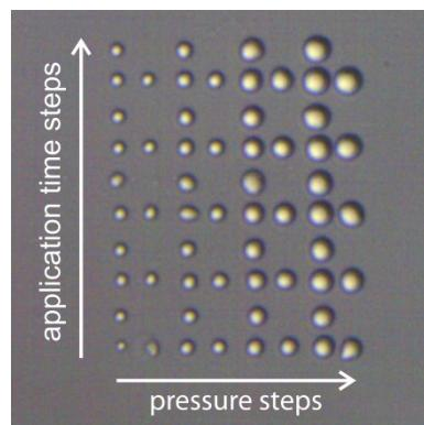
Automated grid calibration varying back pressure (left to right with increasing pressure) and contact time (bottom to top with increasing time). For each condition 3 spots were printed.
