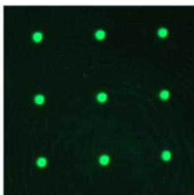
Spotting under liquid environment of Alexa 488 labeled streptavidin on a biotin modified substrate<sup>[1]</sup>
