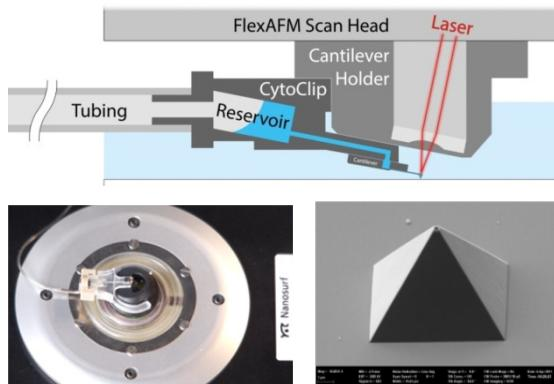
FluidFM probes have a closed channel connecting the cantilever opening to a fluid reservoir. A controller is used to vary back pressure to the reservoir to allow deposition parameterization. Force control is obtained through laser-based measurement of cantilever bending by the AFM that is an integral part of the FluidFM system.
