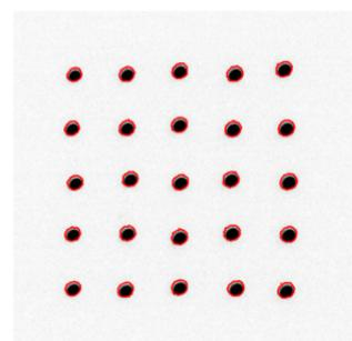
Air environment, 250 mbar back pressure, 1 s contact time. Diameter:  $4.83 \pm 0.17 \mu\text{m}$
