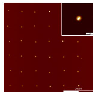
Air environment, 100 mbar back pressure, 50 ms contact time. Diameter:  $615 \pm 60 \text{ nm}$
