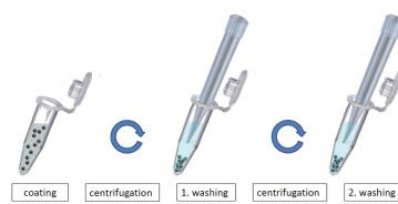
Batch processing of multiple beads: a large reservoir of equally coated beads is accessible.
