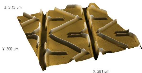
Figure 5: 3D representation of a stitched AFM image. The image (corresponding to the stitching result in Figure 4), shown here at 200-fold magnification, demonstrates how easily high-resolution 3-dimensional data can be acquired using the Nanosurf Nanite B AFM and an automated translation stage. It also demonstrates how seamless the result of the stitching process is.
