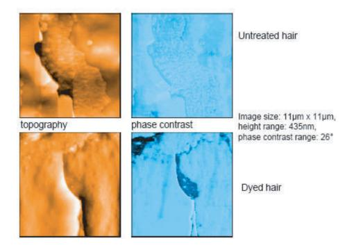
DFM head. The phase mode images were obtained with the modeExtension option. The X-Y table option was used to facilitate positioning of the tip with respect to the hair.
