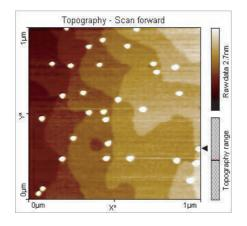
The upper image on the left hand side was measured with the Mobile S AFM using a high resolution scan head. The white particles are 30nm large Q-dots. The mono atomic terraces in the underlying surface are clearly visible and prove the quality of the measurement.
