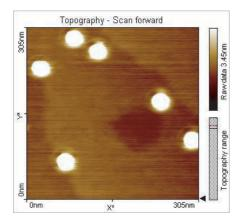
The lower image on the left hand side is a zoom into the previous image. It shows the perfectly round shape of the Q-dots.
