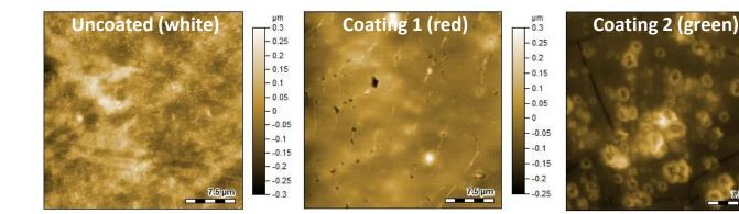
Friction properties from lateral deflection measurements
