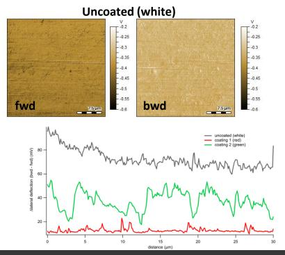
Polymer coating reduces the surface friction of the tubing.
