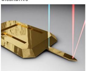
CleanDrive is a photothermal method to actuate the cantilever. Photothermal excitation provides unparalleled stability, and a high excitation bandwidth in air and liquid environments.
