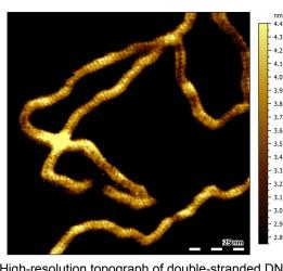
High-resolution topograph of double-stranded DNA (dsDNA) adsorbed to mica in buffer solution. Several dsDNA strands can be observed. All of them show a characteristic periodic pattern.
