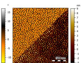
This image shows the phase (top) and topography (bottom) of an unannealed PS-PB-PS triblock copolymer thin film on mica imaged at 20 Hz line rate using an USC-F1.2-k7.3 cantilever.
