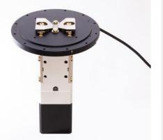
The variable magnetic field sample holder is made for MFM measurements with DC magnetic field applied in-plane with the sample. Areas of application are magnetic imaging of ferromagnetic films and nanostructures. The holder is compatible with the environmental control option.
