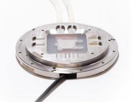
The heater/cooler sample holder is suitable for scanning probe measurements at temperatures above and below ambient. Areas of application are imaging of various phase transitions and electrochemical experiments at various temperatures. The accessory comes with a temperature reference unit and water pump.
