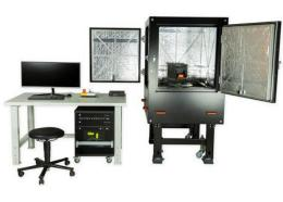
Alphacen 300 is Nanosurf's first large sample AFM system with a fully accessible 300 x 300 mm sample stage. The Alphacen 300 can handle samples with a maximum size of 710 x 710 x 45 mm and maximum weight of 45 kg.
