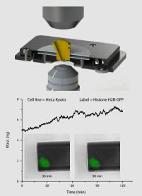
Optical microscope integration and full temperature, gas, and humidity control allow continuous monitoring of cells over a long period of time (up to days) with optical techniques (e.g. DIC, fluorescence) in addition to mass measurements. Images in graph show a time series of Histone H2B-GFP-labelled HeLa cells attached and growing on the Cytomass Monitor's cantilever. Data courtesy Müller lab ETHZ.
