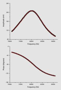
High-quality frequency and phase data are essential for precise mass measurements. This is why the Cytomass Monitor uses photo-excitation of its cantilever. Observe the excellent correlation of experimental data (black squares) and fitted curves (red lines).
