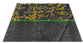
**Figure 3.** In situ AFM image in 1 mM CuSO<sub>4</sub> + 50 mM H<sub>2</sub>SO<sub>4</sub> showing Pt surface covered with electrochemically deposited copper clusters at *E* = -0.05 V (upper part) and bare Pt surface at *E* = 0.3 V (lower part), 3  $\mu$ m × 3  $\mu$ m, vertical range 100 nm. The potential scan was performed at the position of the horizontal green line.
