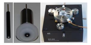
**Figure 1**. Rod-like electrode (left) mounted inside a sample holder (center) and fixed in Electrochemistry Stage ECS 204 (right).
