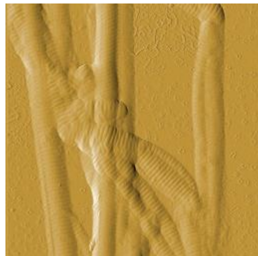
Figure 3. AFM deflection image recorded along with the height image shown before. The D-banding is visible for all fibrils. As expected, fibrils oriented perpendicular to the fast scan axis show weaker contrast in the deflection image.
