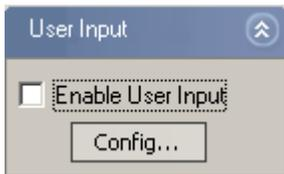
The User Input is available in all imaging and spectroscopy modes except in the "Spreading resistance"-Operating mode. If you click on "Config" you can freely define a name for the user input, define the physical unit of the signal and its range.
